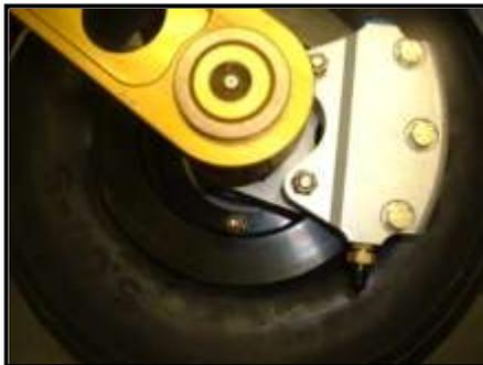
**Note:** Much like your outboard motor it is wise to force out any water in the wheel axle area by filling it with grease. Also wise to ensure no water is in the floats when freezing time starts and even leave covers loose so no condensation collects.
